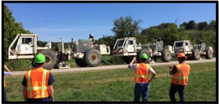
Seismology students observing three vibroseis trucks at a predefined shot point.
