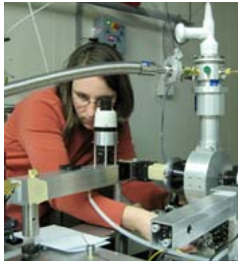
(left) Diamonds in a diamond anvil cell compressing a sample to the pressures of the Earth's deep interior. (Right) Dr Panero aligning a diamond cell at the National Synchrotron Light Source beamline U2A to measure the bonding properties of water in mantle minerals.
