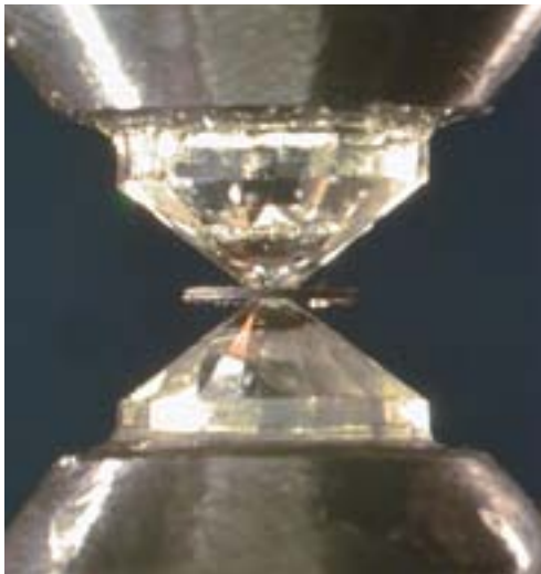
(left) Diamonds in a diamond anvil cell compressing a sample to the pressures of the Earth's deep interior. (Right) Dr Panero aligning a diamond cell at the National Synchrotron Light Source beamline U2A to measure the bonding properties of water in mantle minerals.
