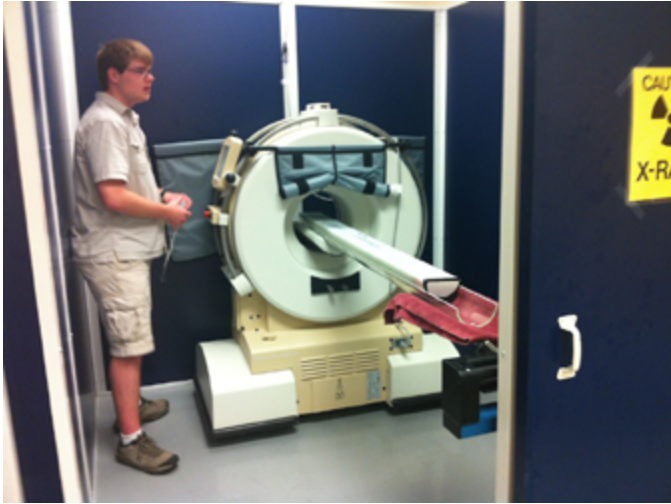
Derek Kackley, SES sophomore, prepping the new X-ray Computed Tomography (XCT) machine to scan an Arctic sediment core from Byrd Polar Research Center.
