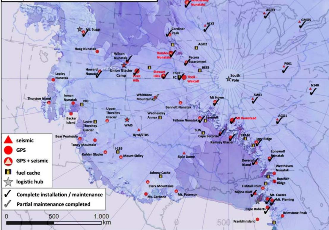
Map of ANET/POLENET GPS & seismic network in Antarctica, superposed over a map of the USA to better illustrate scale. Sites installed this year are labeled in red letters. Sites visited to date marked by a check. Existing sites in West Antarctica were not scheduled for work this season. Field sites were reached by Twin Otter aircraft from hubs at Union Glacier, South Pole and McMurdo Station.
