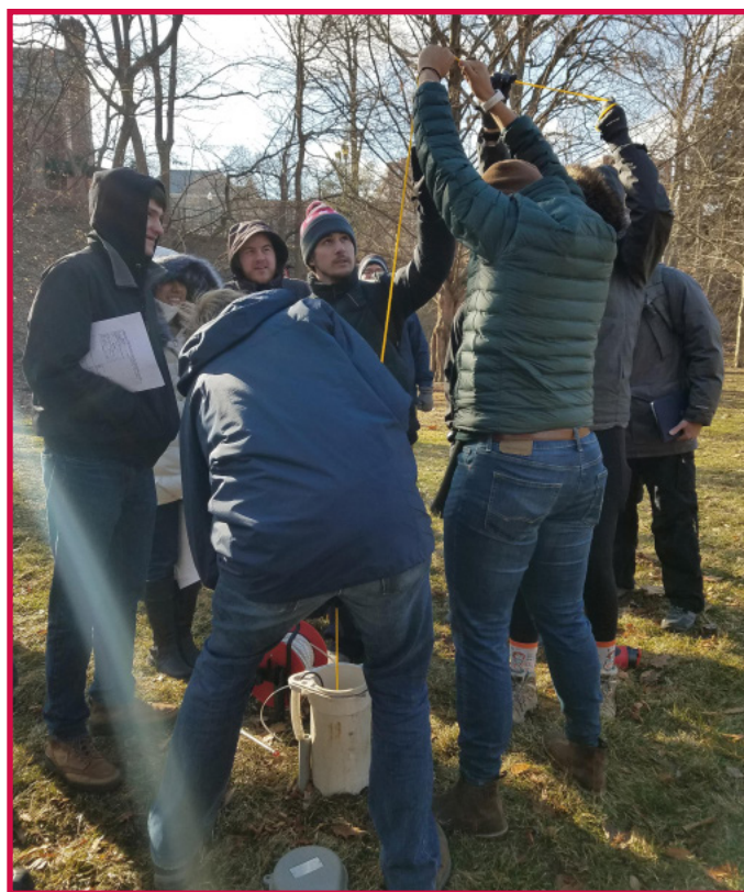
Students in ES 5651 conduct a slug test in the 120-foot groundwater well.
