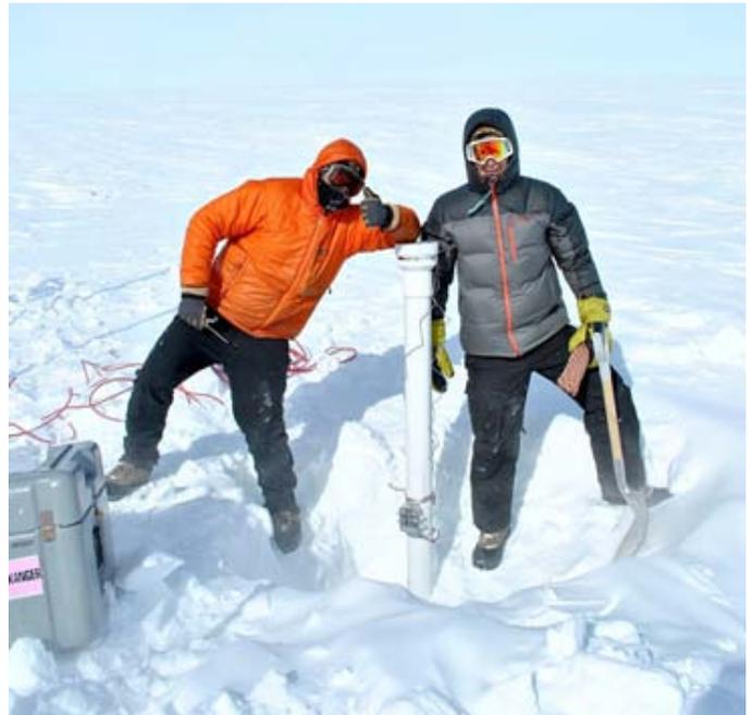
*Howat (left) and Research Associate Dr. Santiago de la Pena (right) installing a snow sensor on the Greenland Ice Sheet to measure the rate of thickness change. Photo by Steve Price.*
